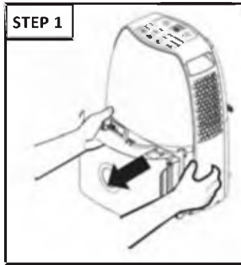
Slide water tank out
